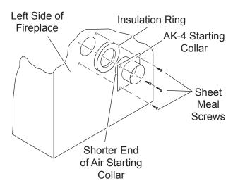
Figure 20 - Attaching Outside Air Starting Collar and Insulation Ring to Left Side of Fireplace
